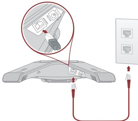
Use the Ethernet cable to connect the **INTERNET** port on the back of the Yealink CP920 IP phone to an available wired Internet connection.
